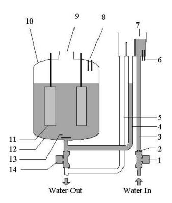
cylinder so periodically the controller will open the drain valve (14) and drain some of the mineral laden water away and replace it with fresh water. If the water rises too high, or foaming occurs, this is detected by the cylinder full electrodes (8).
