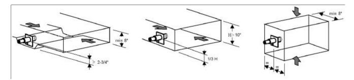
To mount the steam distributor nozzle, cut or drill a 2-1/2" hole in the duct. Apply caulk to the mounting plate of the nozzle. Attach the nozzle to the duct using  $4 \pm 10$  by  $\frac{1}{2}$ " drill point self-tapping sheet metal screws (not supplied). Nozzle must be level with condensate outlet to bottom.
