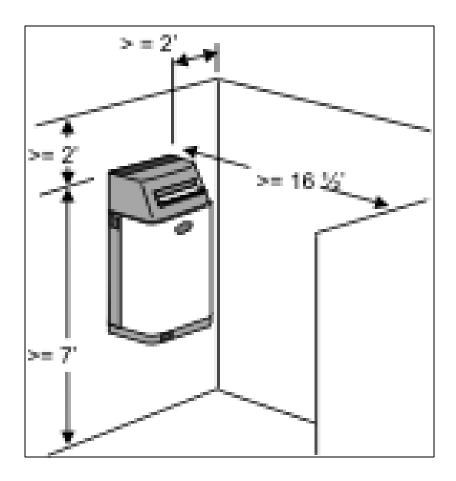
The room distribution unit is used to distribute the steam directly into the room, and is supplied premounted to the top of the humidifier.
