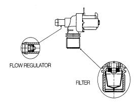
WARNING: When cleaning the fill valve, do NOT poke or probe flow regulator with any object which may enlarge the orifice. The flow regulator must meter water flow precisely or shortened cylinder life may result.
