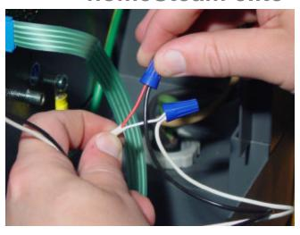
To make the homeSteam elite operate, it is only necessary to complete the circuit between these two wires through the proper controls. The drawing below is the standard wiring.
