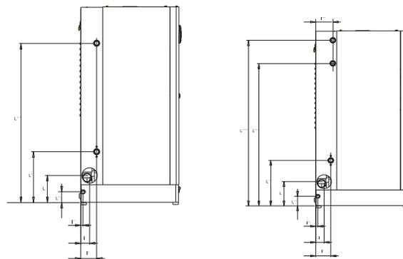
Interfaces dimensions steam outlet and condensed drain
