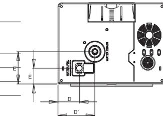
Interfaces dimensions steam outlet and condensed drain
