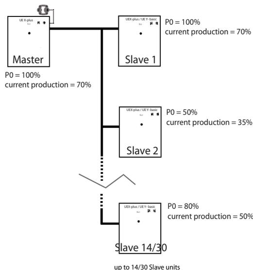
Connection between UEX Master and UEX/UEY Slave. Use shielded cable for the connection.
