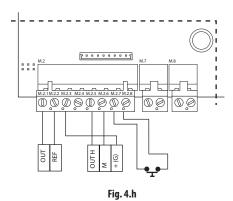
The reference (zero) of the external controller must be connected to the GND terminal (M2.2) and the control signal to terminal M2.1.
