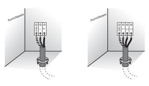
Fig. 4.c (view inside unit, electrical compartment)
