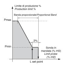
Fig. 14.3 Control with limit probe
