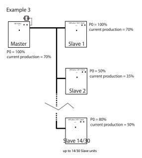
Connection between UEX Master and UEX/UEY Slave. Use shielded cable for the connection.
