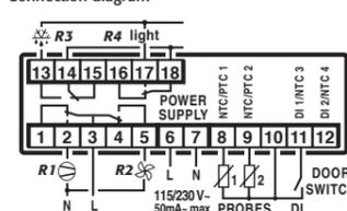
\*: short-circuit terminals 10 and 11 if the door switch is not used
