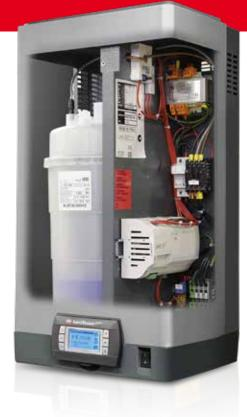
humiSteam operation is based on a very simple physical principle. As common drinking water contains a certain quantity of dissolved mineral salts, and is consequently slightly conductive, applying a voltage to metal electrodes immersed in the water creates an electric current that heats the water until boiling, thus producing steam (Joule effect).
