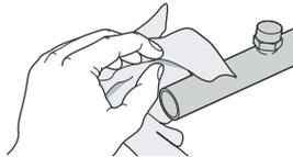
4. Carefully lubricate all contact surfaces.
