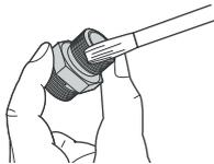
5. Correctly insert the nut and the gasket onto the pipe.
