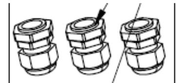
☑️ PG13 cable glands for the electrical connections
