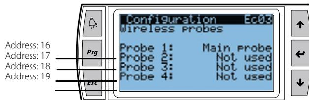
**Note:** the wireless probes are managed on the heaterSteam titanium version.
