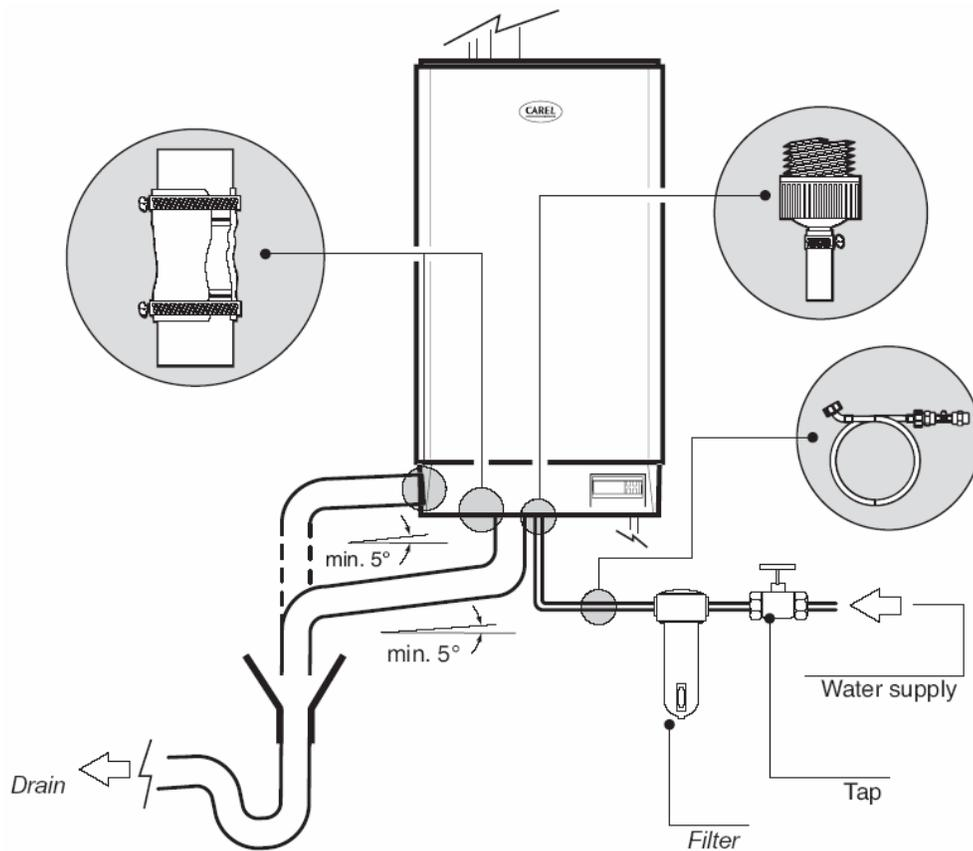
**WARNING: Do NOT use PVC piping unless the unit has the optional drain tempering valve installed.**
