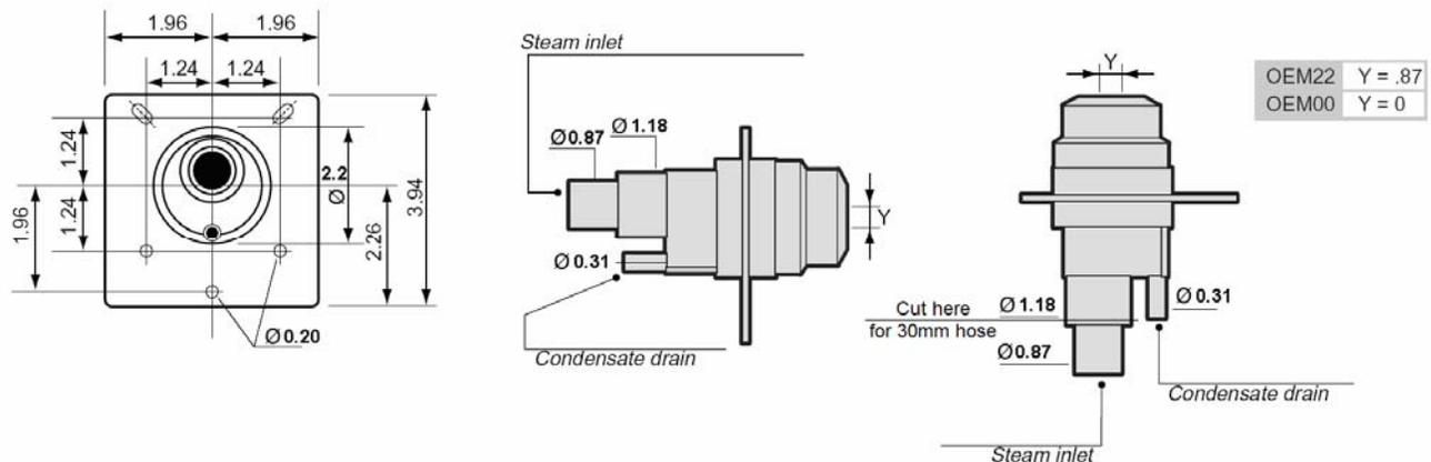
As with the stainless steel distributors, cut a hole in the duct to match the insertion part, apply silicon sealant to the duct mounting plate, fasten with 4 sheet metal screws and connect the steam hose and condensate lines using the hose clamps provided.
