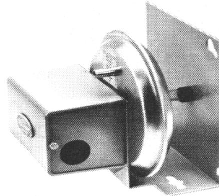
If the airflow switch is to be mounted on the return duct (vacuum), then mount it in a vertical position by the small plate. Drill a 7/16" hole in the side of the duct and connect the supplied tubing to the low pressure tap on the airflow switch and then run it through the drilled hole in the duct. Put no more than 2" of tubing into the duct. Caulk around the tubing where it enters the duct. The high pressure tap is left open to atmosphere.
