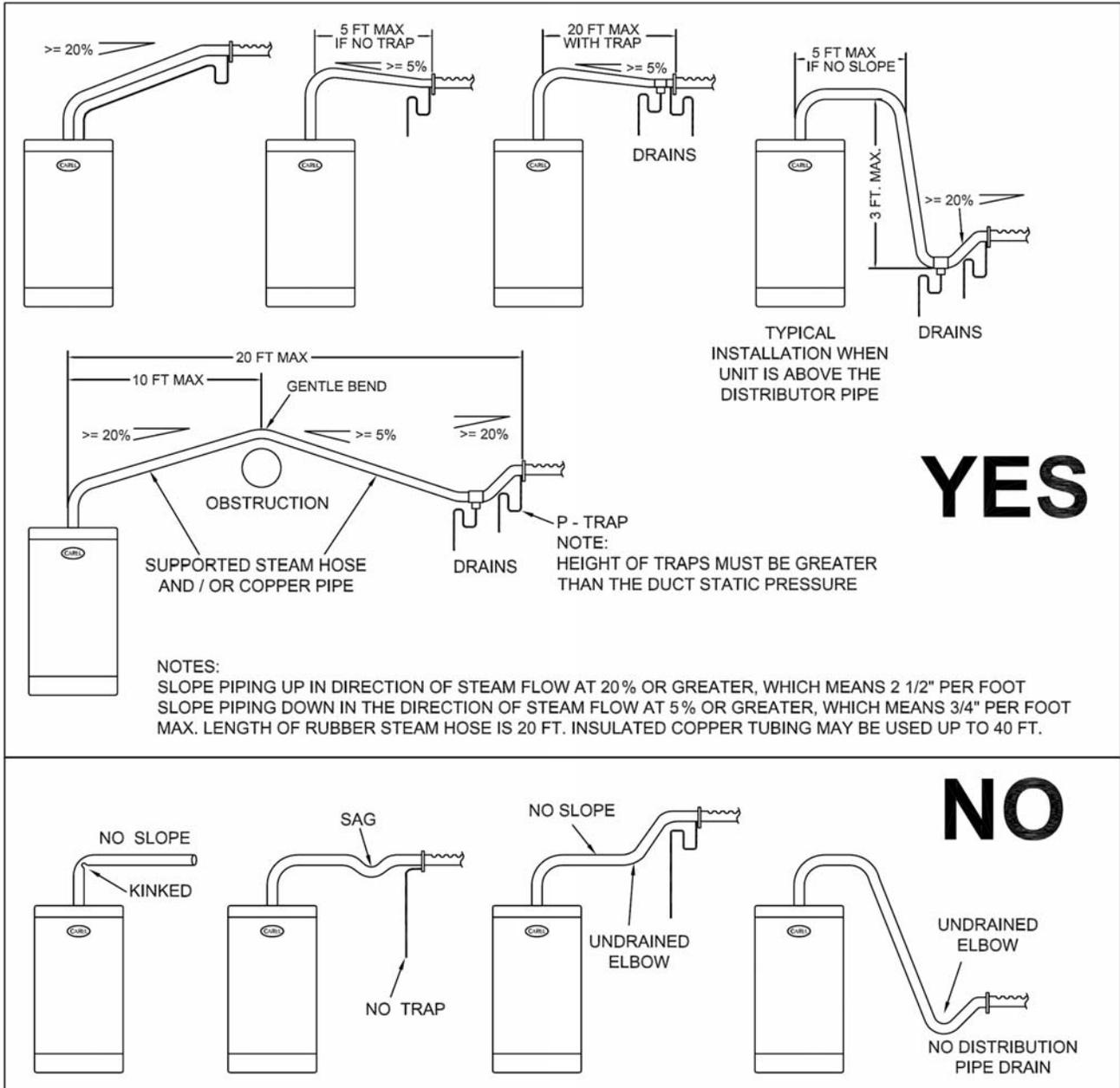
**IMPORTANT: Maximum length of rubber steam hose is 20 feet. Insulated copper tubing may be up to 40 feet. In all cases, minimize sharp bends and elbows – use 2-45° elbows instead of 90°s.**
