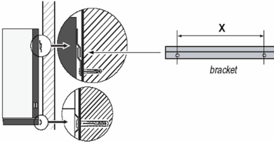
Once the mounting bracket is secured to the wall, hang the unit on the bracket. Fasten the remaining capture screws through the bottom holes in the unit to secure it to the wall.
