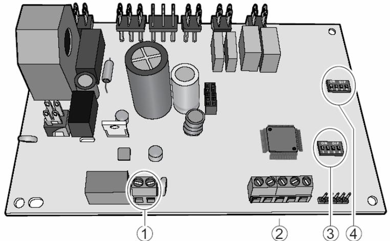
Control Signal Terminal Block (# 2 in diagram)
