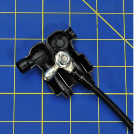
Step #4: Torque down bolt to 3 N/M while holding spark plug adaptor on 90 degree angle from cylinder power cable.
