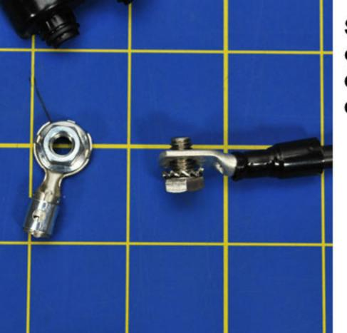
Step #2: Slide lock washer onto bolt and insert through existing cylinder power cable end.
